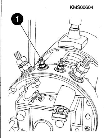
Detach all other connections at starting-motor solenoid (1) and control relay (2).
